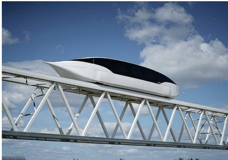
Fig. 2 – Intercity passenger SkyWay vehicle – a high-speed (up to 500 km/h) 6-seat family-type unibus
