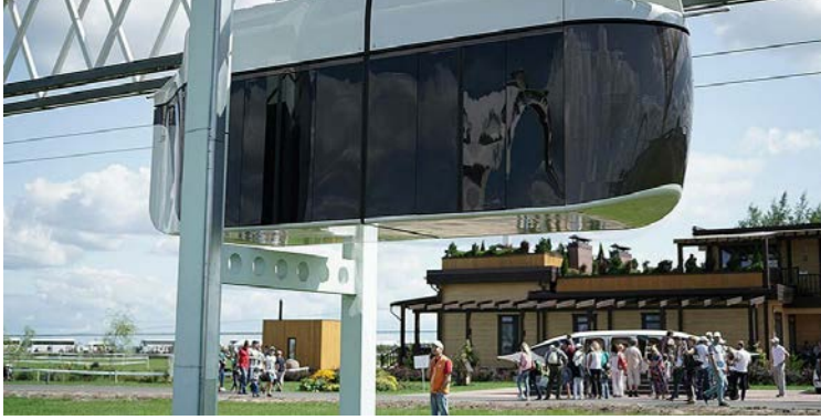
Fig. 1 – Urban passenger SkyWay vehicle – a suspended quad-rail 48-passenger unibus, Maryina Gorka, 2019
