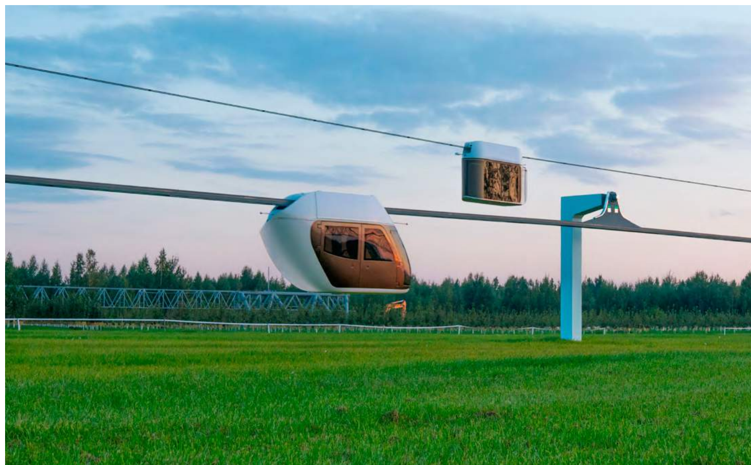
Samples of SkyWay transport rolling stock unibus and unibike at running tests in the demonstration and certification center of the developer-Company EcoTechnoPark (Minsk region, 2017)
